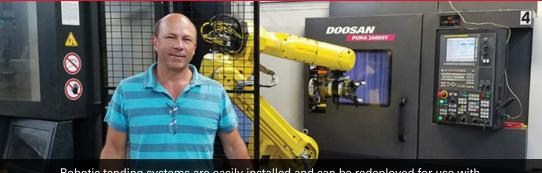
Robotic tending systems are easily installed and can be redeployed for use with other equipment.
