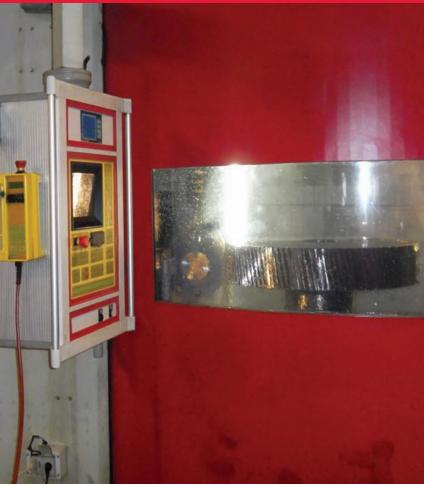
**Left**: A gear blank being turned on PEM's You Ji Vertical Lathe by machinist Brian Oman. **Right**: PEM's Hofler Rapid 2000 Geargrinder cutting teeth into the gear blank.
