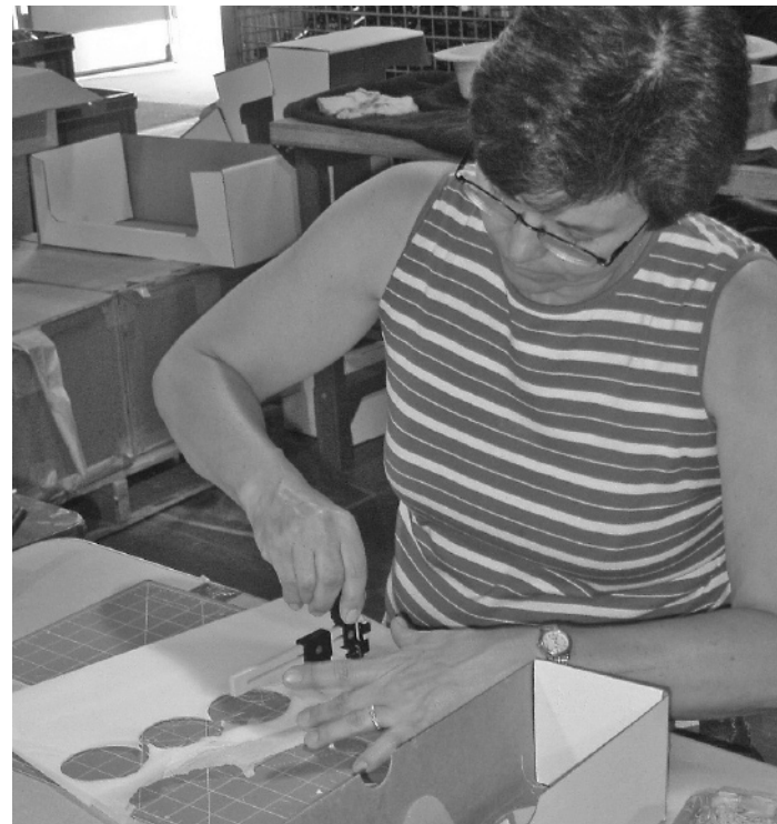
Goodwill’s contracts supervisor, Nancy Feldmann, shown above manually cutting filters used in the deer repellent product assembly.
