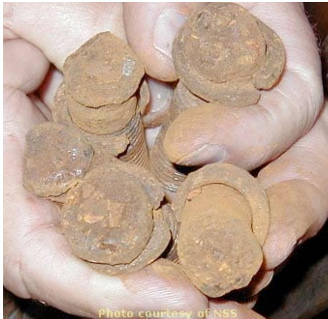
**Figure 7.19** Impeller and bowl bolts from the tower water pump evaluated by PSAT in Figure 7.18
