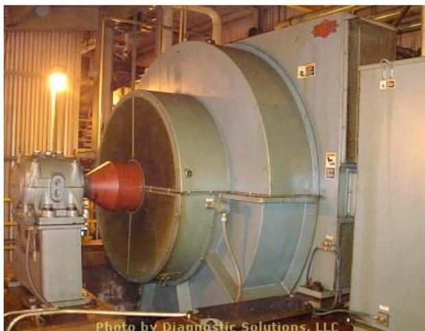
**Figure 7.8** Synchronous 3850-hp Motor
