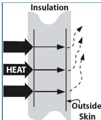
**Figure 4.9** Heat Losses through Wall<sup>32</sup>
