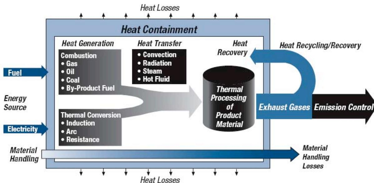
**Figure 4.3** General Schematic of a Typical Process Heating System<sup>22</sup>
