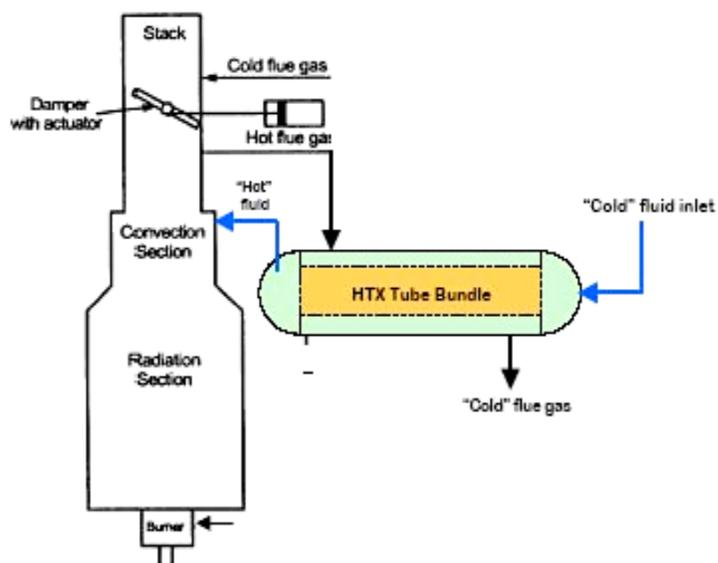
**Figure 4.12** Typical Load Preheating System Using Exhaust Gases
