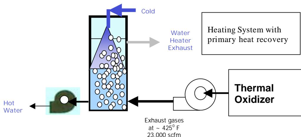
**Figure 4.14** Typical Direct Contact Water Heater Systems
