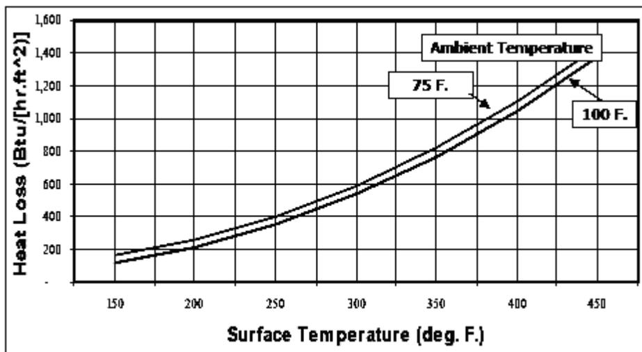
**Figure 4.10** Chart for Estimating Wall Heat Losses
