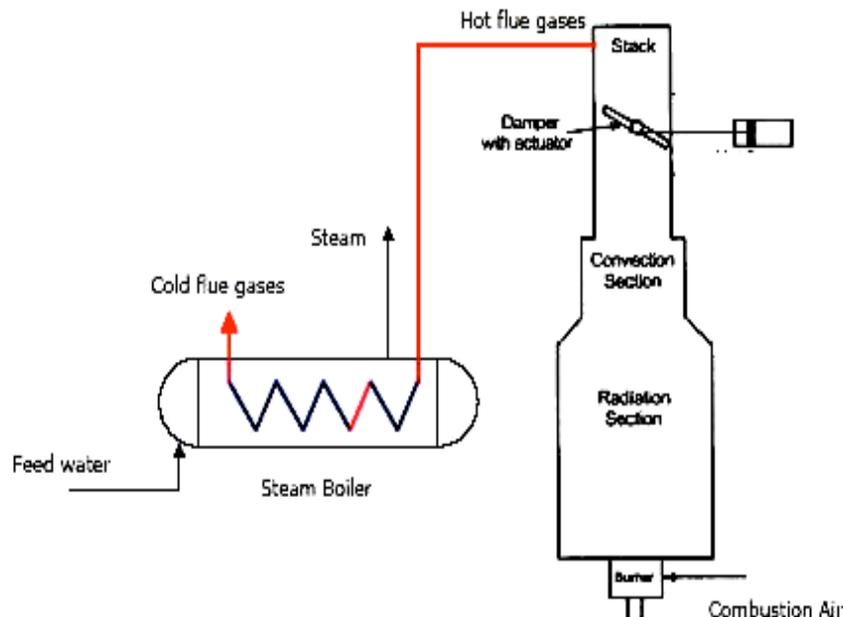
**Figure 4.13** Typical Waste heat Boiler Steam generation System
