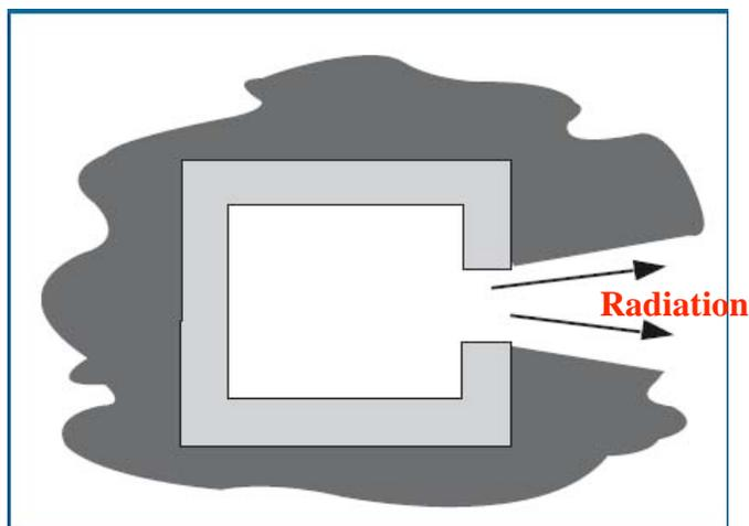
**Figure 4.11** Radiation Heat Losses from an Opening<sup>33</sup>
