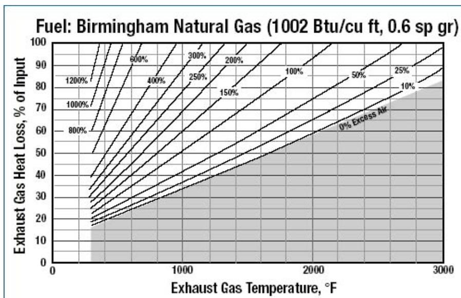
**Figure 4.5** Exhaust Gas Heat Losses vs. Exhaust Gas Temperature<sup>27</sup>
