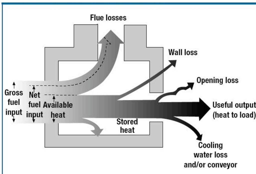
**Figure 4.4** Schematic Indicating Heat Losses in a Generic Process Heating Application<sup>26</sup>
