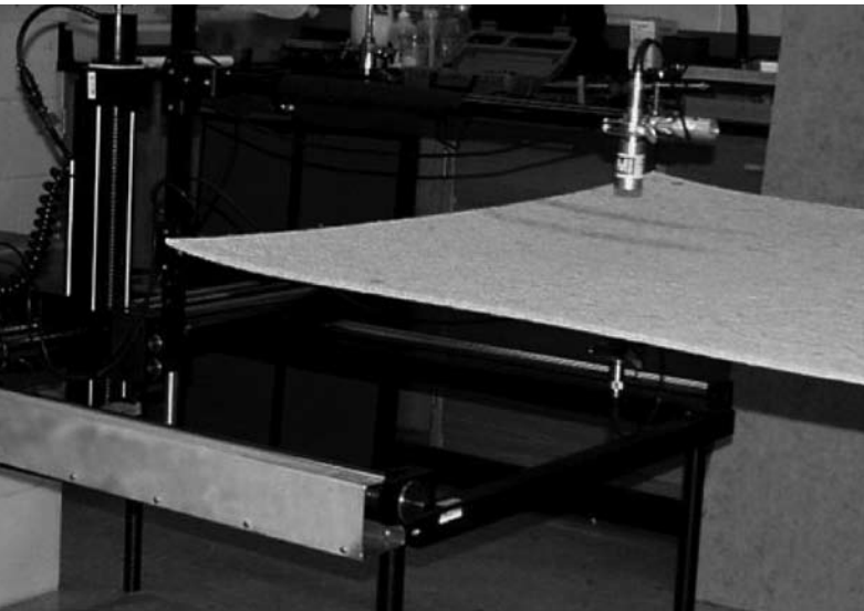
Figure 1: Air-coupled ultrasonic transducers are scanned over kenaf-reinforced panels.
