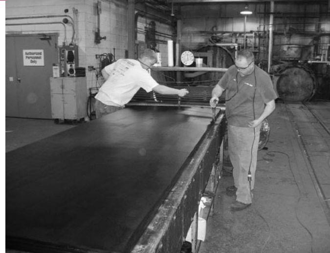
Employees trimming rubber on a plate prior to being placed in a vulcanizer
