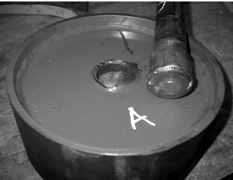
Failure of a large pulley brought the Chantland Company of Humboldt, Iowa, to IPRT for help with discovering its cause. The pulleys are used in applications such as baggage handling equipment in airports.
